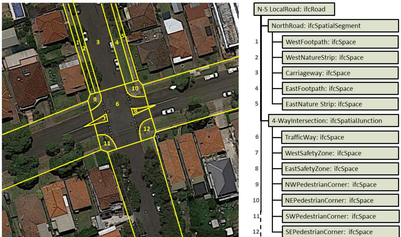
Figure 31 - Typical 4-way local road junction showing a spatial decomposition of one road segment and the intersection
